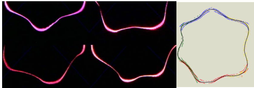
Fig. 5. Four pictures of a cross section curves and the reconstructed cross section
